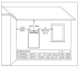
• At least 500 mm between the flue terminal and a fence, wall or other obstruction, in the direction of the flue discharge.
