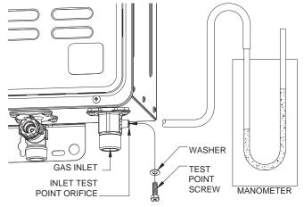
5. Observe the gas pressure reading on the manometer.
