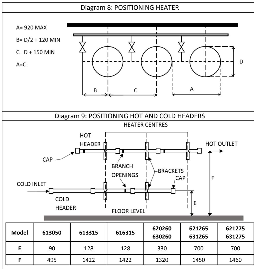
6. Silver solder header joints and end caps. It may be convenient to install the gas manifold at this stage.
