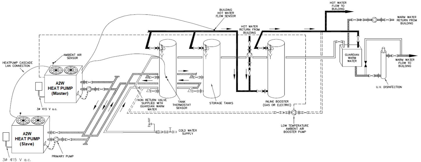
**Typical A2W Heat Pump Installation with Inline Boost, Low Ambient Air Boost
