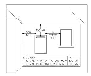
• At least 500 mm between the flue terminal and a fence, wall or other obstruction, in the direction of the flue discharge.
