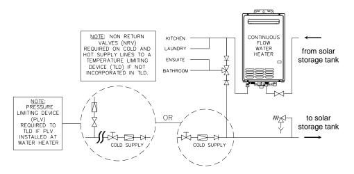
Gas Booster for Closed Circuit Indirect Solar Preheater Installation Two Temperature Zones Using a Temperature Limiting Device
