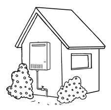
The water heater must not be installed in an area with a corrosive atmosphere where chemicals are stored or where aerosol propellants are released. Remember the air may be safe to breathe, but when it goes through a flame, chemical changes take place which may attack the water heater.
