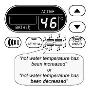
During Step 6, when the BATH FILL button is pressed to turn the Bath Fill mode on
