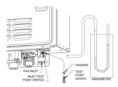
If the manometer reading is between the minimum and maximum inlet gas pressure ratings on the rating label, no adjustment is required.
