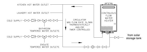
NOTE: A PLV IS REQUIRED TO BE INSTALLED ON THE COLD SUPPLY LINE TO THE TEMPERING VALVE IF A PLV IS INSTALLED ON THE COLD SUPPLY LINE TO THE WATER HEATER.
