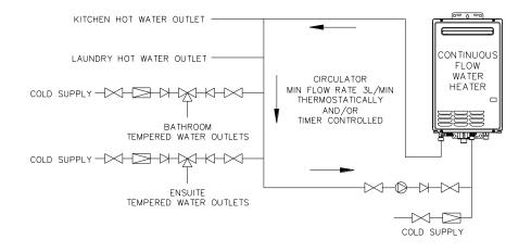
NOTE: A PLV IS REQUIRED TO BE INSTALLED ON THE COLD SUPPLY LINE TO THE TEMPERING VALVE IF A PLV IS INSTALLED ON THE COLD SUPPLY LINE TO THE WATER HEATER.
