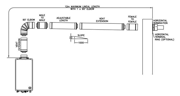
Typical Installation – Horizontal Terminal with One Bend
