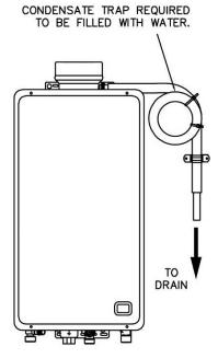
**Condensate Trap and Condensate Drain Line**
