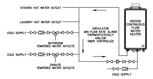
NOTE: A PLV IS REQUIRED TO BE INSTALLED ON THE COLD SUPPLY LINE
