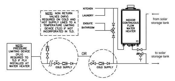
In-series Gas Booster as part of a Closed Circuit Solar Water Heater Installation
