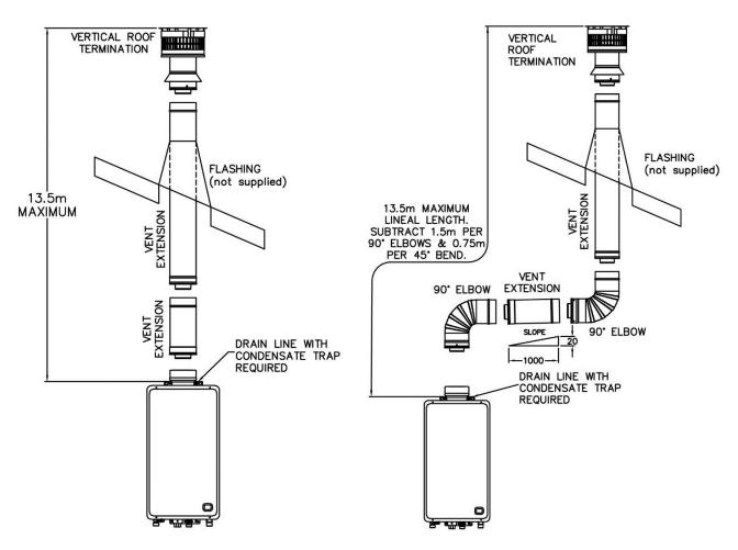
Typical Installation Vertical Flue
