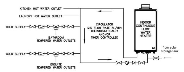
NOTE: A PLV IS REQUIRED TO BE INSTALLED ON THE COLD SUPPLY LINE
