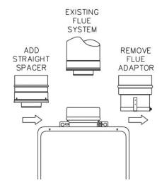
Remove Flue Adaptor – Install Straight Spacer
