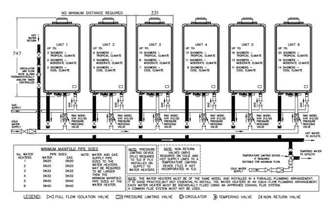
**Note:** An isolation valve and pressure limiting valve are not required on the solar preheat water line to the gas boosters as part of a solar water heater installation. A full flow isolation valve must still be installed on the inlet branch of each water heater.
