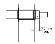
19. Apply an adequate bead of sealant around the flue assembly and exterior wall of the building, using a general purpose silicone sealant suitable for outdoor application.
