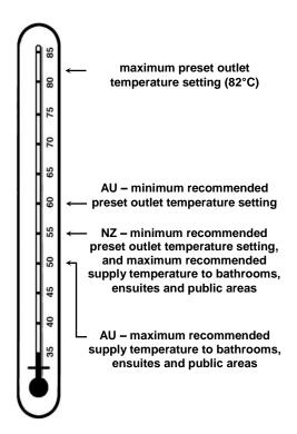
**Note:** Australian Standard AS 3498 and New Zealand Building Code Clause G12 requires that a water heater provides the means to inhibit the growth of Legionella bacteria in potable water. When this water heater is used as an in-series booster for a solar water heater it can satisfy these AS 3498 and Clause G12 requirements provided it is energised, the booster preset outlet temperature setting is 70°C or higher, and that a remote temperature controller is not used.
