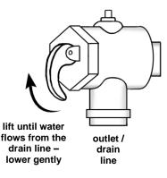
Operate the easing lever on the temperature pressure relief valve and expansion control valve once every six (6) months to clear any deposits and ensure the valve and its drain line are not blocked. It is very important the lever is raised and lowered gently. Refer to "Minor Maintenance Every Six Months" on page 29.
