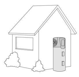
The water heater must be installed with a clearance of at least 25 mm from a wall behind the water heater. To maintain the designed performance, air flow and air discharge from the heat pump, the minimum distances to a wall or obstruction from the water heater and measured horizontally along the wall are:
